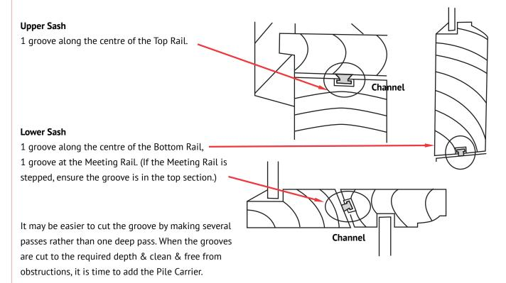
Measure the length of groove, allowing 10mm extra. Remove backing tape and insert into groove, making sure Pile Carrier is flush with the end of the groove. Trim any excess overlap Insert Weatherfin Pile into the Pile Carrier and trim to length. Secure with small pins if necessary, use a nail punch to ensure they are flush.
